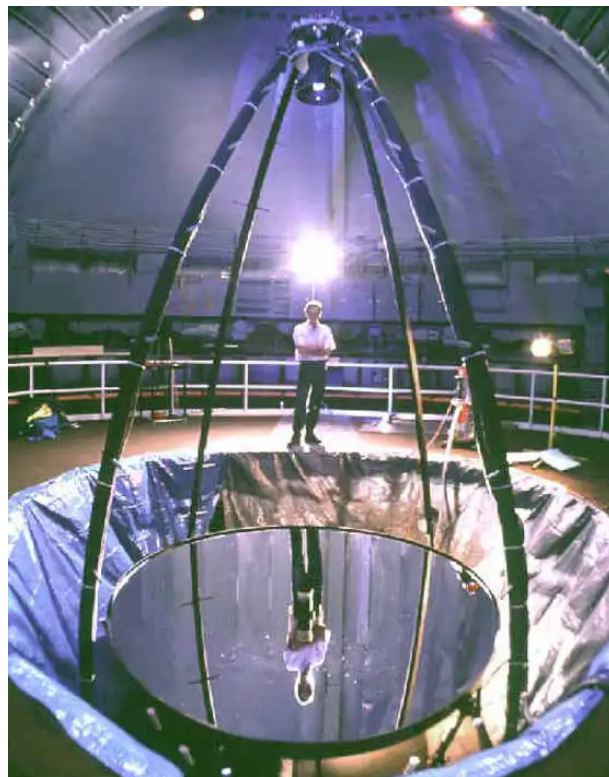
Fig. 1: Liquid-mirror telescope at NASA Orbital Debris Laboratory.
